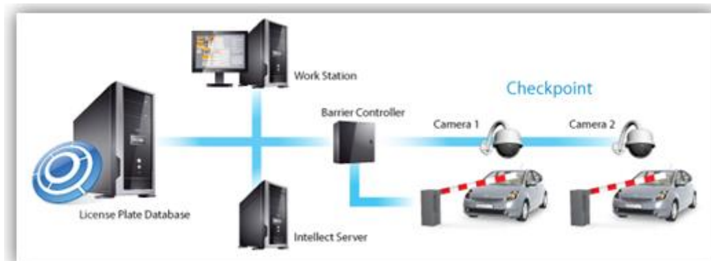
Figure 14 License Plate Recognition (FidPark, 2017)
